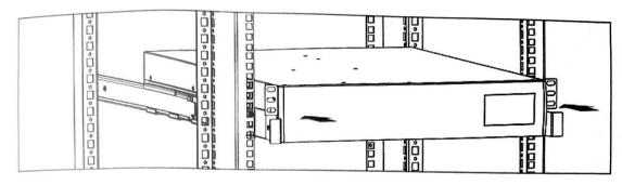
Step 5: Fix the UPS in position with 4 screws.
