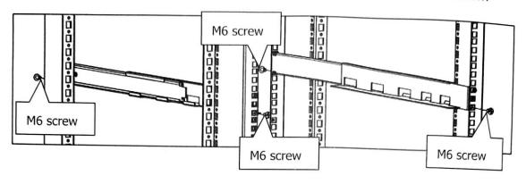
Step 3: According to UPS height, put 6 pieces of nuts on proper location.
